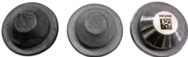
Left: Forged part with data matrix code, middle: after sand-blasting, right: machined part with laser code.
